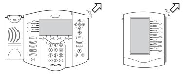
(2) Align the Expansion Module at the top of the groove lines on the SoundPoint<sup>®</sup> IP 601 phone and slide unit downwards until unit clicks into position. Connect the Base Stand for each Module.
