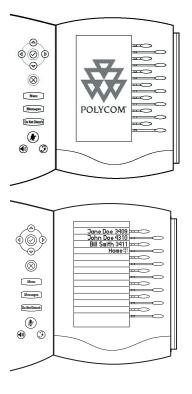
Power is automatically transferred from the host SoundPoint<sup>®</sup> IP 601 phone to Expansion Module(s) upon connection. Units may be plugged and unplugged (hotswapped) at any time to a live SoundPoint<sup>®</sup> IP 601 host phone.
