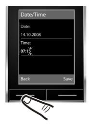
▶ Press the key below Back on the display screen to return to idle status.
