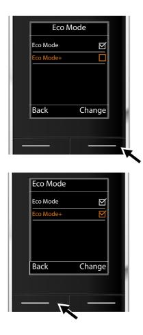
Press down on the control key until the Eco Mode+ menu option is highlighted.
