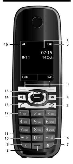
Illustration of handset on a base with SMS functionality.
