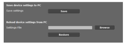
Once you have configured the DECT Manager and after making any changes to the configuration, particularly registering or deregistering handsets, you should save the latest settings in a file on the PC so that the current system can be restored quickly if problems occur. The file is stored with the suffix .cfg (default: Gigaset-yyyy-mm-dd.cfg).
